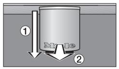
Pull the main dispenser all the way down ① and pull the cover forward to remove ②.
